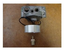
Remove the original filter bowl and its sealing ring (which may be stuck in the filter head). If fitted, remove the splash plate (this looks like a large steel washer) in the centre of the filter head. If there is a felt washer under the plate remove this also. Fit the large sealing ring supplied into the groove in the filter head.
